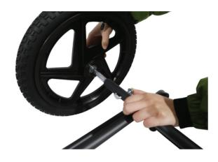
3) Assembly of drawbar remove safety pin from trailer bar under the trailer, and extend it. Put safety pin back to lock bar.
