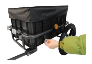
On Your Bicycle: Unscrew the rear axle nut, install the towing hitch and secure the nut; extend the trailer bar, line up and connect the front end to the towing hitch on the bike. Secure the pin and, for added safety, wrap the harness around the frame.
